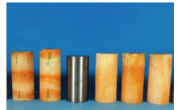
Salt samples after triaxial extension tests
