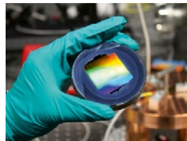
Silicon metasurface for application as a highly reflective mirror in the near infrared spectral range.
