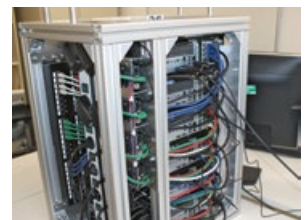
Research prototype for software defined vehicle network (TSN)
