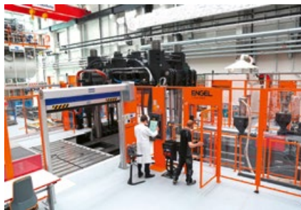
In the large-volume injection molding process, molten plastic is injected at high pressure into a mold in which the component forms its shape. In such a mold, metal inserts, local fiber reinforcements or organic sheets can also be overmolded to hybridize and functionalize the component in the process. © OHLF/Wecke
