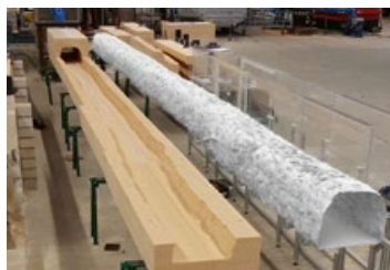
Scale model production of an unlined rock blasted tunnel (white structure shows the digital elevation model of the tunnel). Source: R. Eikenberg
