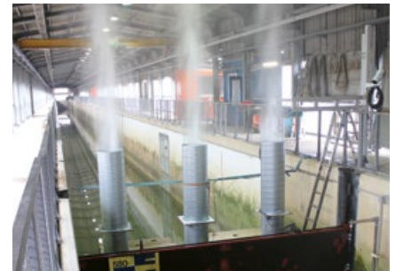
Test of an OWC wave energy converter
