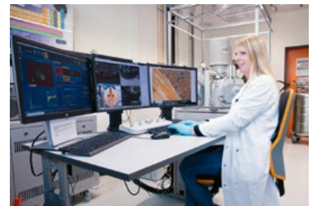
For the purpose of studying the interactions in the manufacturing processes and the analysis of hybrid composite components, the surface structure of materials can be imaged and analyzed down to the nanometer and subnanometer range in the imaging laboratory, equipped with versatile and high-resolution microscopes. © OHLF/Christo
