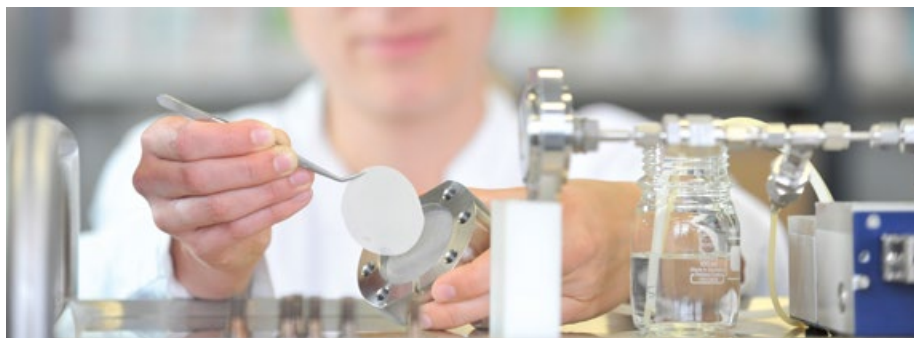
Manufacturing of colloidal drug carrier systems by premix membrane emulsification.
