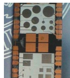
thin-film capacitors fabricated from ZrO 2 nanocrystals
