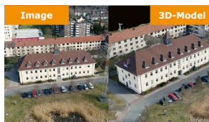
To create geometric (three-dimensional) models out of image sequences is one of the tasks of Photogrammetry. The images in this case were taken by a UAV.
