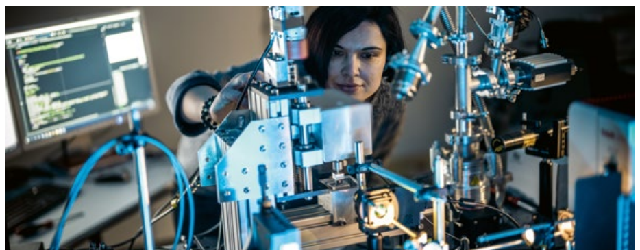
LENA High-End analytical Infrastructure – High resolution optical polarimeter for semiconductor material characterization. AG Kroker/IHT, © J.Hosan/TU Braunschweig
