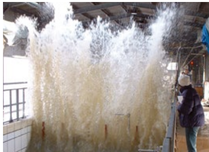
Breaking wave impacting a vertical seawall
